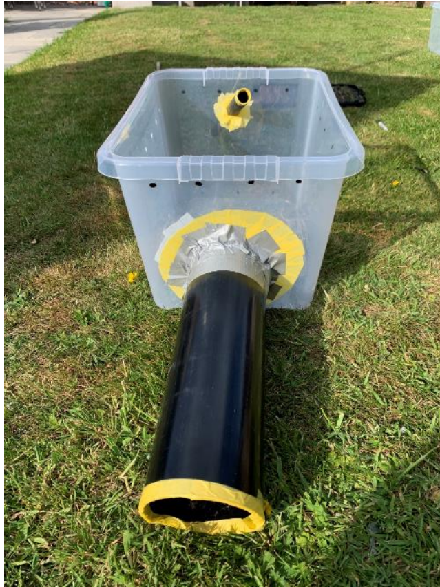
Tunnel attached to main box using duct tape
